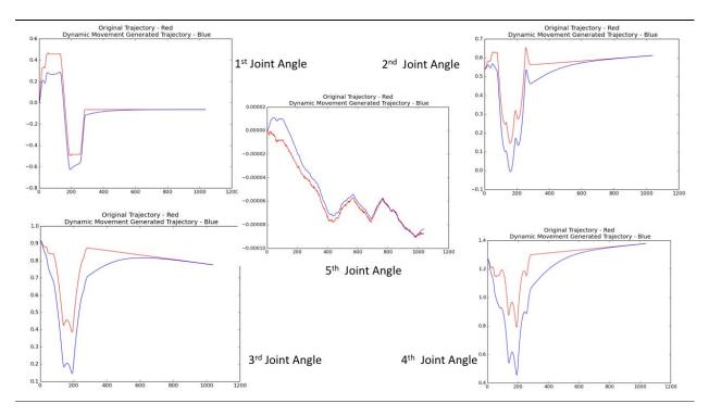
The second case involves changing the end goal. An offset in the values of the joint angles is added to the learned system. The graph shows that even after the step input, the robot is able to adjust its position to match the new goal, even after an offset is given the general trajectory is followed by the learned system.
